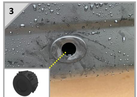
Insert the Parking sensor bungs into the OEM carriers to blank off the holes in place of the OEM Sensors. The bungs push in from the outside.
