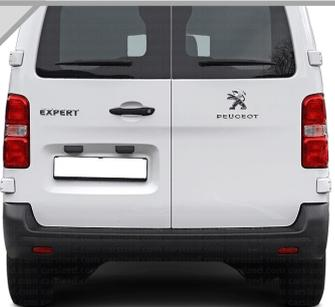
If required remove the bumper to gain access to the reversing sensors.
