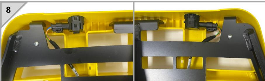
Short Cable on the inner channel of the tread
