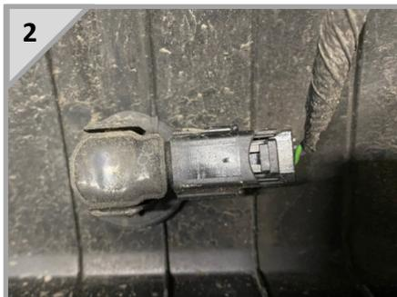
Remove the 4 OEM parking sensors from the rear bumper, leaving the carriers in the bumper.
