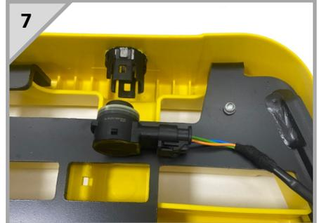
Connect the extension cables to the OEM sensors.
