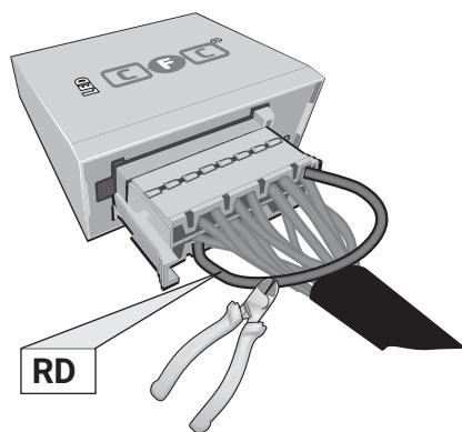
Pin 11 and Pin 2 disconnected
