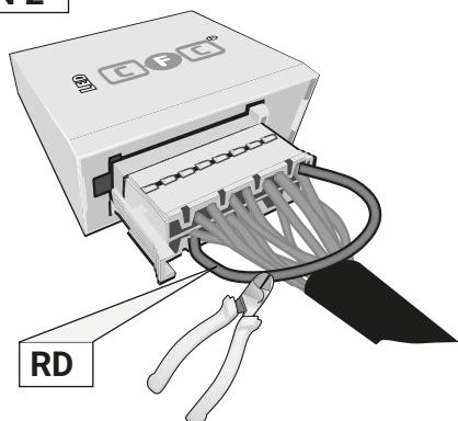
Pin 11 and Pin 2 disconnected
