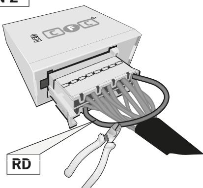
Pin 11 and Pin 2 disconnected
