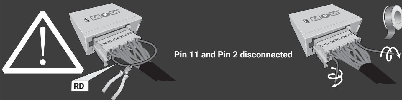
Pin 11 and Pin 2 disconnected
