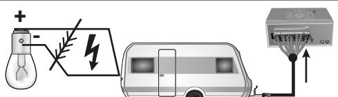
**Short circuit fault on PIN 11, 12 or 14**
