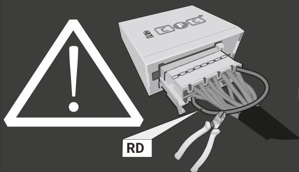
Pin 11 and Pin 2 disconnected
