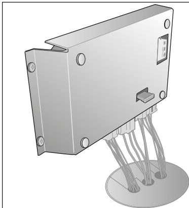
**Start to route the wiring loom from the location of the Sargent VLM7- or VLM5 module.**
