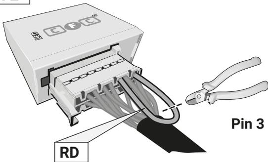
Pin 3 and Pin 2 disconnected
