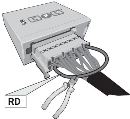
Pin 11 and Pin 2 disconnected
