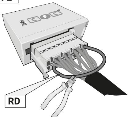
**Pin 11 and Pin 2 disconnected**
