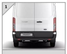
If required remove the bumper to gain access to the reversing sensors.
