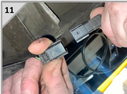
Connect the parking sensor cables to the original vehicle parking sensor connectors and use the larger cable ties to secure in place.
