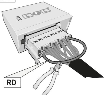
Pin 11 and Pin 2 disconnected
