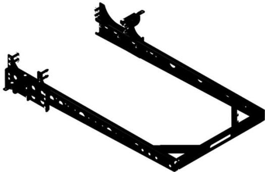
PSA / FIAT MOTORHOME Requires chassis extensions to be fitted to the OEM External face and chassis extensions cut down more than 400mm
