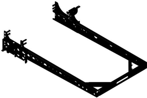
FORD MOTORHOME Requires chassis extensions to be fitted to the OEM External face and chassis extensions cut down more than 400mm
