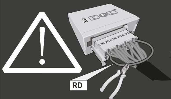
Pin 11 and Pin 2 disconnected
