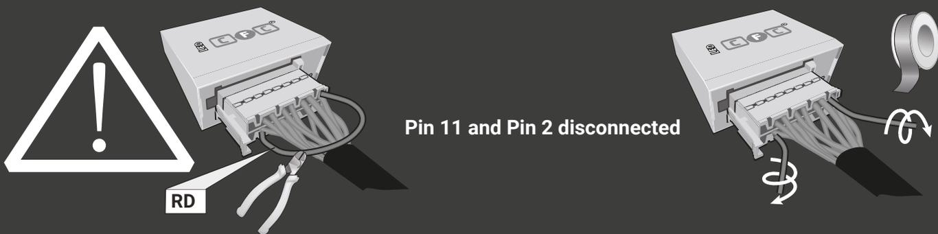
Pin 11 and Pin 2 disconnected
