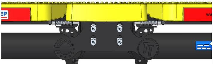
Always ensure central tread is level with the outer treads. Using the remaining fixings bolt your desired ball bracket to the face plate and torque all fixings to 252 Nm
